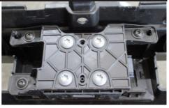
Remove plastic cover, squeeze clips in and remove.
